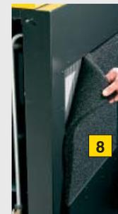
standard high-efficiency coolers provide maximum cooling resulting in approach temperatures as low as 11°F for more moisture separation at the compressor discharge and better air quality. A filter mat simplifies cooler maintenance. Dirt and dust build up on the outside of the filter, where it is easily seen and removed. This extends cooler service intervals and increases thermal reserve for harsher conditions.
