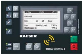
The Sigma Control 2 has a communications port adaptable to Profinet, Devicenet, Profibus, and Modbus for seamless integration into master control/monitoring systems. An Ethernet port with built-in web server enables remote viewing.
