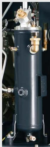
centrifugal action and a 2 stage coalescing filter to reduce fluid carry over to 2 ppm or less. Quick release fittings, drain, and fill ports are arranged for fast and easy fluid changes from sump and cooler without any pumping device. The easy-to-read fluid level indicator can be checked without opening or stopping the compressor through a window in the service panel.
