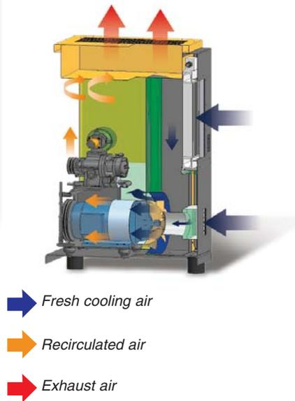
*The SX unit can be installed in a corner and it will still provide easy access for maintenance while allowing for proper cooling air flow.*
