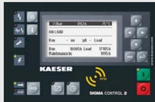
Sigma Control 2 has superior communications capabilities. An Ethernet port and built-in web-server enable remote access. ModBus, Profibus, Devicenet and other industrial communications interfaces are also available as plug in options for seamless integration into plant control/monitoring systems. See our Sigma Control 2 brochure for details.
