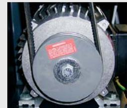
cooled (TEFC) motors with Class F insulation are standard for long life in harsh environments.
