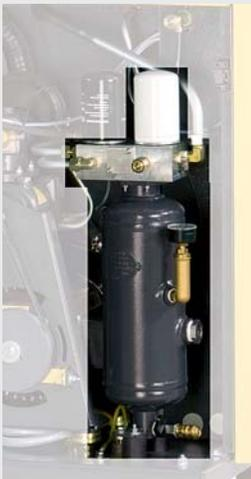
We combine an over-sized cyclone separator vessel (ASME or CRN) with a convenient spin-on coalescing filter for superior fluid separation and exceptionally low carry-over (3 ppm or less). This results in less maintenance and better downstream air quality.
